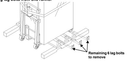
8. Remove the runner from which all lag bolts have been removed (refer to Figure 6).
